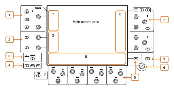
**Preamp** – Peak indicator and dedicated preamp controls for analogue Gain, Digital Trim, 48V, Pad and polarity.
