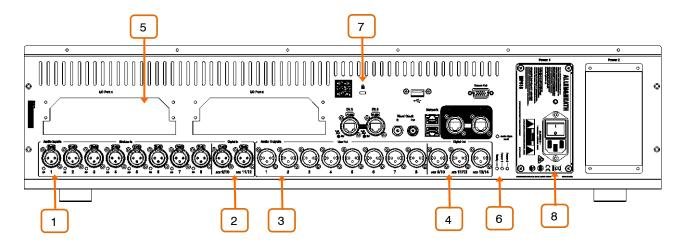
**Mic/Line inputs** – 8x recallable preamps for balanced or unbalanced microphone and line level signals. Gain, Pad and 48V are digitally controlled within the preamp.
